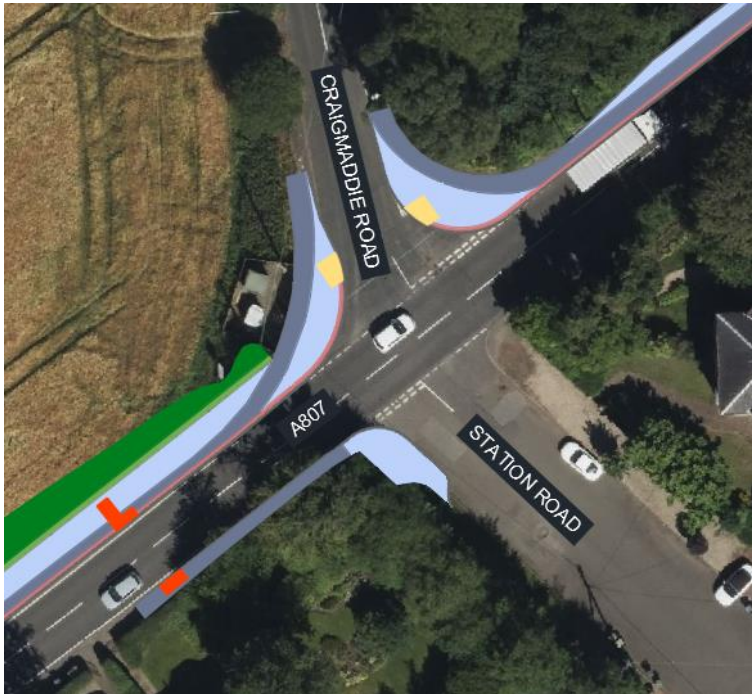
Figure 2.9 – Signalised toucan crossing and junction improvements at the east end of Bardowie
