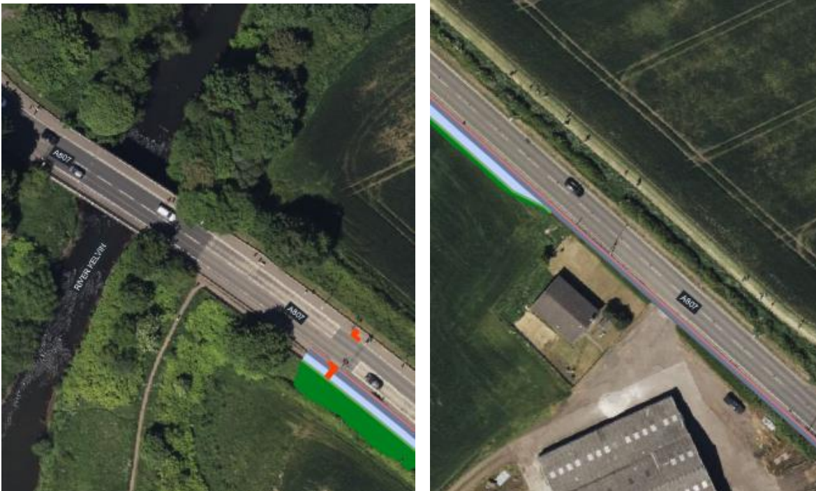
Figure 2.12 – Width constraints over River Kelvin bridge crossing (left), and residential and commercial properties (right)
